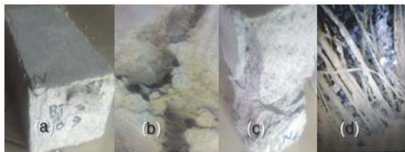
Figure 4: (a) The test object is still intact after a compressive strength test, (b) Fiber palmyra does not break when the test object is destroyed, (c) The test object without using fibers being crushed when testing the compressive strength, (d) Fibre still intact after 6 months of the test object is destroyed.
