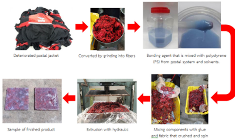
Figure 2: Shows the process of converting into solid sheet material by mechanical thermoforming Source: Teerapong Poti (2020)
