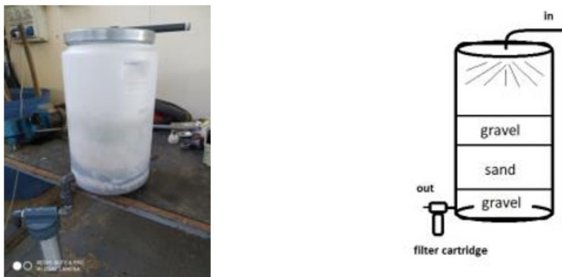
Figure 1: Homemade sand filter and construction scheme
