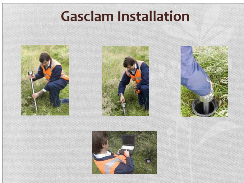
Figure 2: Process of Gasclam installation
