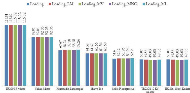
Figure 4: Line loading after optimization process
