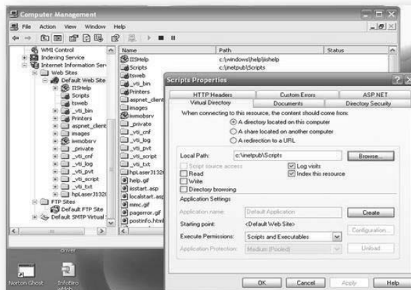
Figure 5. Web Site and Web service enabled
