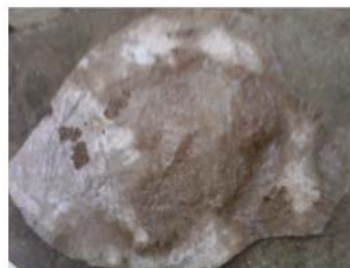
Figure 1b. Photographic Plate of Untreated Blend (0.5g Wood flour / 1 g Polyethylene Loading)
