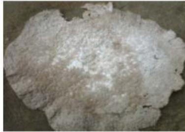
Figure 1a. Photographic Plate of Acetylated Blend (1 g Wood flour / 1 g Polyethylene Loading)
