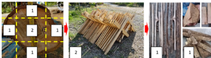
Figure 2: Teak logs obtained from the cutting phase: Part of the Wing of Teak and Part of Teak Source: Author
